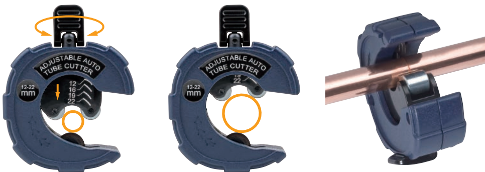
Adjust knob to desired size indicator, insert tube and rotate for auto feed cutting
